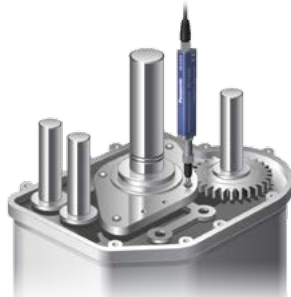
Installed height measurement
