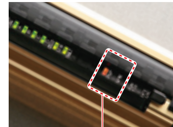
PNP / NPN polarity indicator Either PNP or NPN side lights depending on which is selected.
