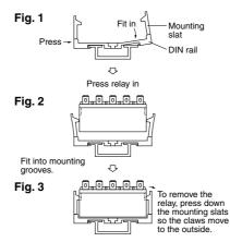
(1) First fit the arc shaped claw of the mounting slat into the DIN rail.
