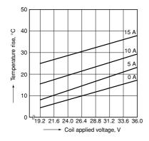
1.-(2) Coil temperature rise (4 Form C type) Tested sample: SP4-DC24V Ambient temperature: 27 to 29°C 81 to 84°F
