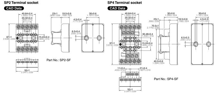
Note: Terminal number marking is on the socket body. Please refer together with the SP relay schematic.
