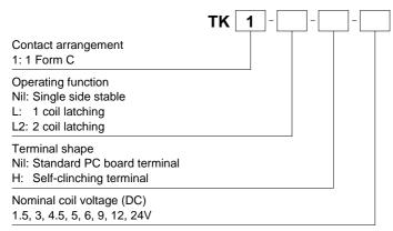
Note: In case of 5 V drive circuit, it is recommended to use 4.5 V type relay.
