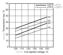
7. Ambient temperature characteristics Tested sample: TX2-5V, 5 pcs.
