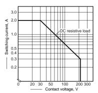
4. Electrical life (2A 30V DC resistive load) Tested sample: TX2-5V, 6 pcs.
