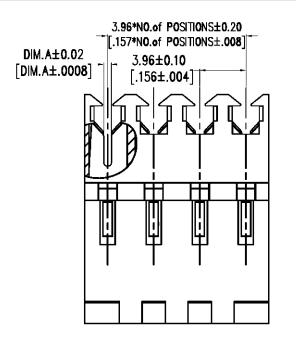
Current Rating: 5.0-8.0 AMP Voltage Rating: 300V AC Contact Resistance: 10mΩ Max
