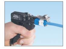
Wire cap and jack module are assembled with additional cycle.
