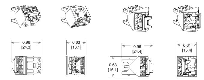
Up/Down 45° Shielded TG Wire Cap CJSUDCAPBU-X, CJSUDCAPIW-X, CJSUDCAPRD-X (See Installation Instruction PN630) Left/Right 45° Shielded TG Wire Cap CJSLRCAPBU-X, CJSLRCAPIW-X, CJSLRCAPRD-X (See Installation Instruction PN629)
