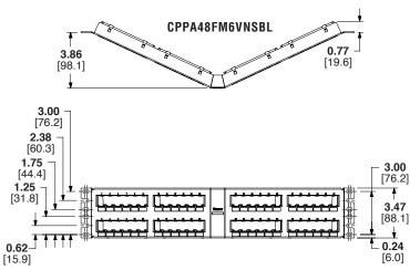
\* White patch panels do not include the write-on detail box below the ports. Dimensions are in inches. [Dimensions in brackets are metric].
