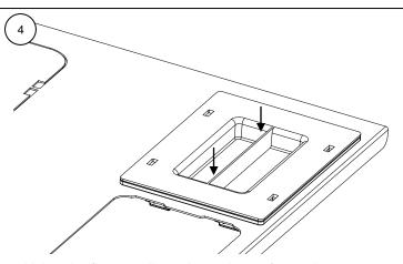
Using the finger pull, apply moderate forces in any direction to ensure the part is secured into the cabinet top cap.
