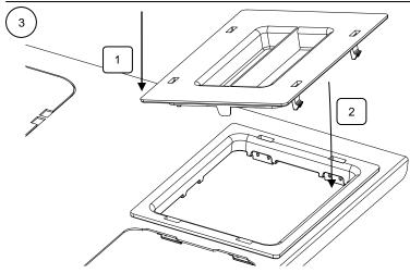
Insert one side of cover, lengthwise, into bezel. Then pivot second side down, snapping cover into place
