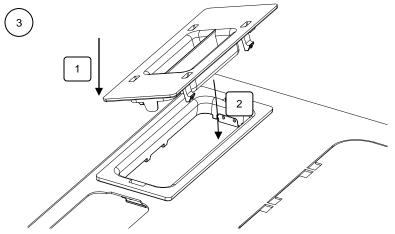
Insert one side of cover, lengthwise, into bezel. Then pivot second side down, snapping cover into place inside bezel.
