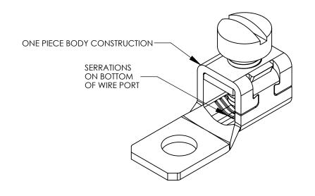
\* MULTIPLE WIRES MUST BE TWISTED TOGETHER BEFORE INSERTION INTO CONNECTOR
