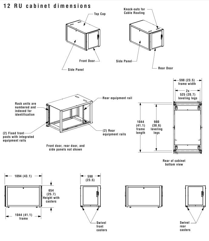
Dimensions are in metric. (Dimensions in parenthesis are in inches)
