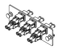
6 POSITION DUPLEX LC FIBER ADAPTER PANEL CUSTOMER DRAWING
