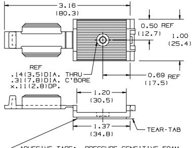
ADHESIVE TAPE: PRESSURE SENSITIVE FOAM 0.040 (1.02) THICK WITH RUBBER ADHESIVE AND PROTECTIVE LINER. MOUNT IS DESIGNED TO SUPPORT 0.62 lbs. (281g) MAXIMUM WEIGHT ON A CLEAN, DRY, SMOOTH, GREASE-FREE SURFACE.
