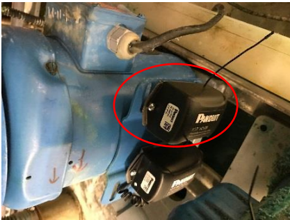
Figure 8: Sensor Magnetically Mounted to Equipment
