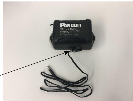
Figure 11: Temperature Sensor with Extended Lead Routed Through Curl on Universal Mount
