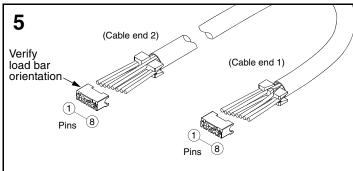
· Orient load bar with contact slots facing downward.
