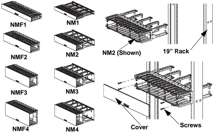
Install the managers to the rack with 12-24x1 screws provided. Install the Covers to the manager by positioning it flat against the front/rear of the manager and pushing to snap in place.
