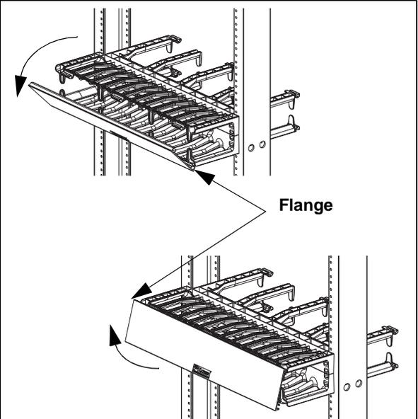
The hinged cover opens from the top or the bottom. Pull flanges to open and push cover to close.
