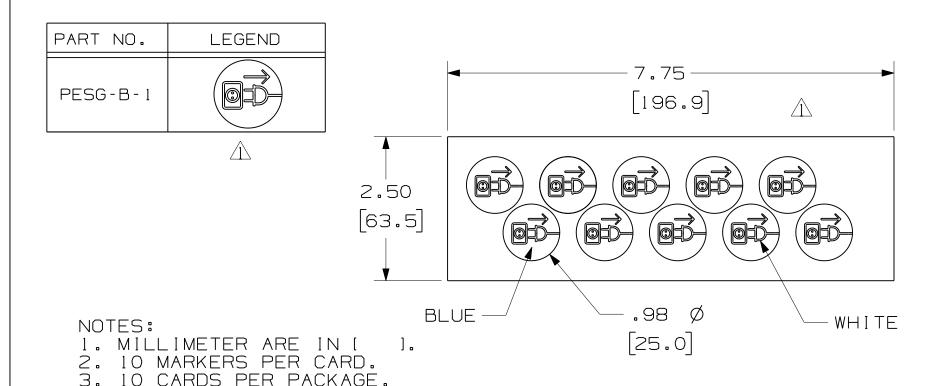
CAD FILENAME/LAYERS 100318MA\_DS\_C10659/00B CORP. TINLEY PARK, ILLINOIS CUSTOMER DRAWING PESG-B MANDATORY SIGNS UNLESS OTHERWISE SPECIFIED, UNLESS OTHERWISE SPECIFIED. DIMENSIONAL TOLERANCES ARE: ALL DIMENSIONS ARE GIVEN (.X) ± .1 (.XXX) ± .025 (.XX) ±.050 ANGLES ± 5° IN INCHES, THIRD ANGLE PROJECTION. MAT'L; 10/21/09 JHAC 5885 R REMOVED WHITE CONTRAST CIRCLE RVU DATE DRAWING NO. GMV1-OL R 7/21/08 RVU DRAWING RELEASE 5361 7/21/08 VINYL FILM C10659
