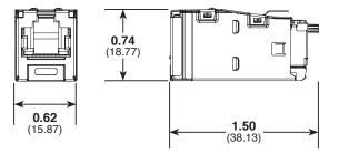
Dimensions are in inches (Dimensions in parenthesis are metric)
