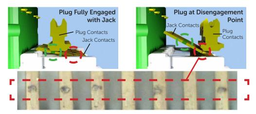
Figure 1: Minor arcing (red) does not occur in Panduit jack mating region (green). Non-Panduit jacks may see such damage in the critical mating area.
