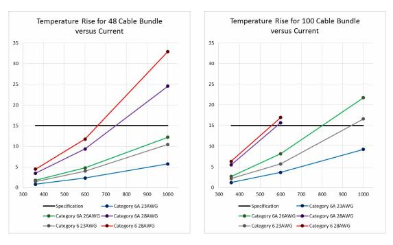
Figure 3: Bundle Temperature Rise over Time for 48 and 100 Cable Bundles
