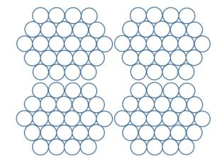
Acceptable deployment of 96 cables using four 24 cable bundles carrying 71 W / 960 mA over Category 6A 28 AWG
