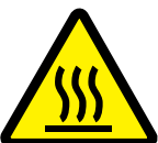
W3198 Heated/Hot Surface Hazard
