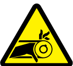
W3154 Belt Drive Entanglement Hazard
