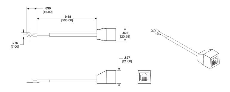
Dimensions are in inches. [Dimensions in brackets are metric].
