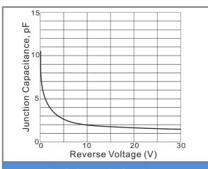
Fig.2 Typical Junction Capacitance
