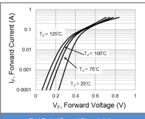
Fig.4 Typical Forward Characteristics
