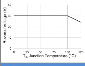
**Fig.5 Operating Temperature Derating Curve**
