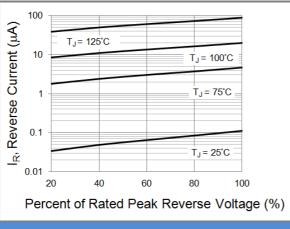
Fig.3 Typical Reverse Characteristics
