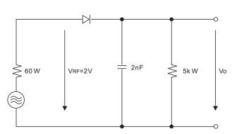
RECTIFICATION EFFCIENCY MEASUREMENT CIRCUIT
