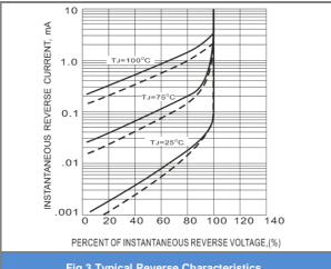
Fig.3 Typical Reverse Characteristics
