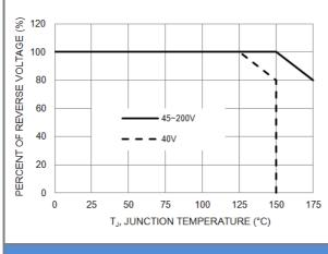
**Fig.5 Operating Temperature Derating Curve**
