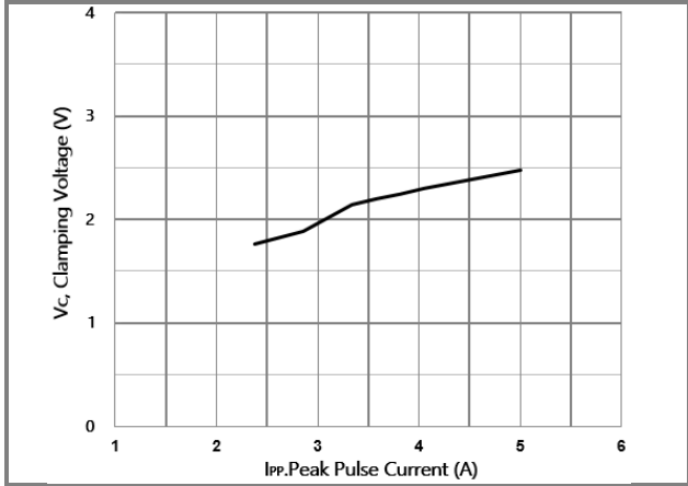
Fig.1 Typical Peak Clamping Voltage
