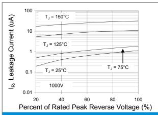
Fig.4 Typical Reverse Characteristics
