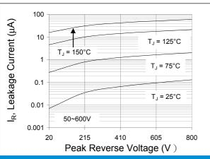
Fig.3 Typical Reverse Characteristics
