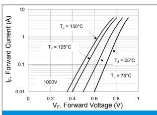
**Fig.6 Typical Forward Characteristics**
