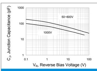
Fig.2 Typical Junction Capacitance
