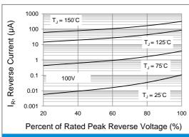
**Fig.5 Typical Reverse Characteristics**
