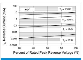
Fig.4 Typical Reverse Characteristics
