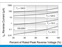
Fig.6 Typical Reverse Characteristics
