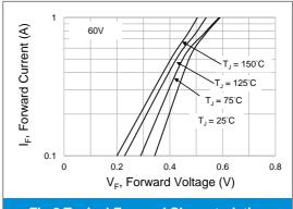
Fig.8 Typical Forward Characteristics
