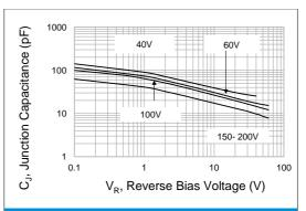
Fig.2 Typical Junction Capacitance
