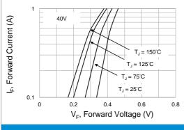
**Fig.7 Typical Forward Characteristics**
