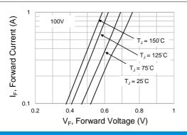
**Fig.9 Typical Forward Characteristics**
