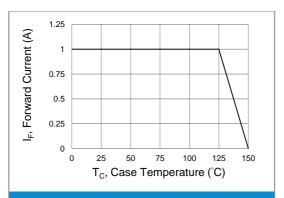
**Fig.1 Forward Current Derating Curve**
