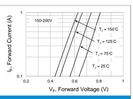
**Fig.10 Typical Forward Characteristics**
