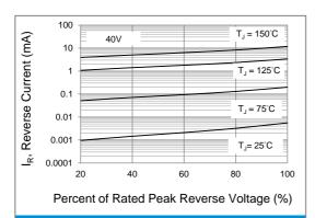
Fig.3 Typical Reverse Characteristics
