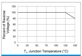
**Fig.11 Operating Temperature Derating Curve**
