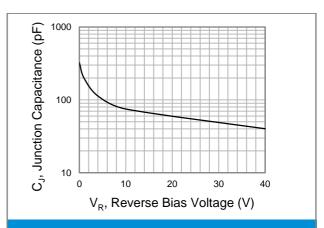
**Fig.2 Typical Junction Capacitance**
