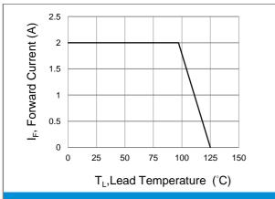
**Fig.1 Forward Current Derating Curve**
