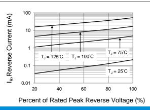
**Fig.3 Typical Reverse Characteristics**
