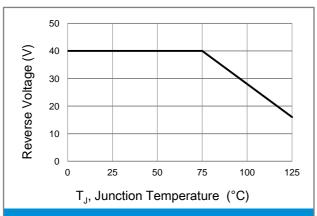
**Fig.5 Operating Temperature Derating Curve**
