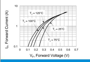
**Fig.4 Typical Forward Characteristics**
