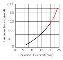
Fig.3 Luminous Intensity vs.Forward Current
