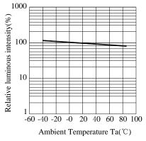
Fig.5 Luminous Intensity vs. Ambient Temperature
