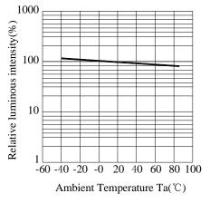
Fig.5 Luminous Intensity vs. Ambient Temperature
