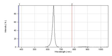
Fig.1 Red Relative Intensity vs. Wavelength
