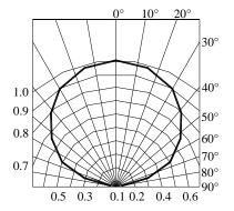
Fig.7 Relative Intensity vs.Angle
