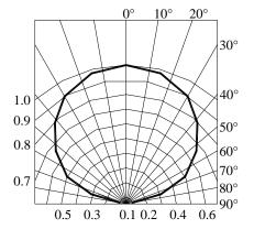
Fig.7 Relative Intensity vs.Angle
