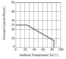
Fig.6 Forward Current Derating Curve
