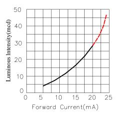
Fig.3 Luminous Intensity vs.Forward Current
