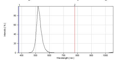
Fig.1 Green Relative Intensity vs. Wavelength
