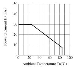
Fig.6 Forward Current Derating Curve
