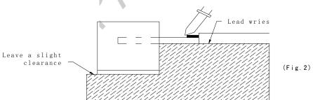
Regarding solution in the tinhing oven for product-tinhing, compound sub-solution made of tin & copper and sliver is proposed with the temperature of Celsius 260. The proportion of the alloyed solution is tin 95.5: copper 3.5: silver 0.5 by percentage. The time of tinhing is constantly 3 seconds.
