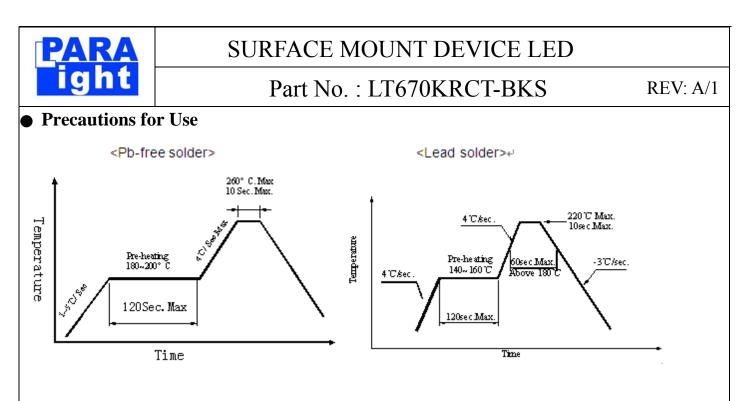
Reflow soldering should not be done more than two times
