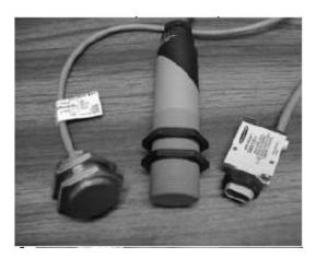
**Figure 3-20** Inductive, Capacitive and Optical Proximity Switches
