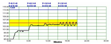
With a K<sub>P</sub> of 0.1, temperature stabilized several degrees away from the setpoint. With bias at 50%, the proportional drive had to be positive to drive temperature up. But the
