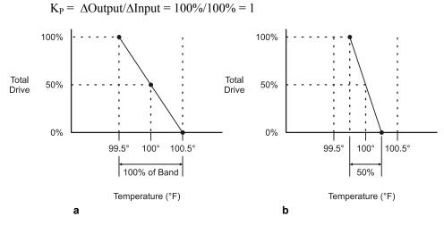
Figure 8-14: 100% Proportional Band (a) and 50% Proportional Band (b)
