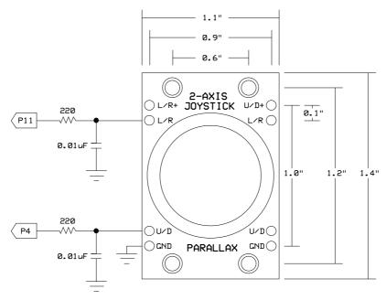
This circuit works with the code below for the BASIC Stamp 2 to provide an RCTIME value for each axis that relates to the position of the joystick. In this manner the two potentiometers are providing a variable resistance for use with the RCTIME command. **Caution:** When using this circuit, do not use a resistor value less than 220  $\Omega$  and do not apply more than 5 VDC through this resistor to the L/R or U/D pins.
