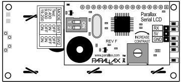
As you can see from the table, there is also a fourth choice called Test. Use this Test mode to confirm that the power and ground to the LCD are hooked up correctly before you send it any data. Move the dip switches to the Test setting and turn on the power. The LCD display should turn on with the backlight on (models 27977, 27979) and display the following text:
