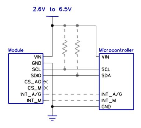
The SDIO and SCL pins also support I2C communications. The pins have internal 100 kilo-ohm pull-up resistors, but external resistors may optionally be used for longer runs or higher speeds. The accelerometer, gyroscope, and temperature sensor have a 7-bit I2C slave address, in hexadecimal, of 0x6A, and the magnetometer has a7-bit I2C slave address, in hexadecimal, of 0x6A.
