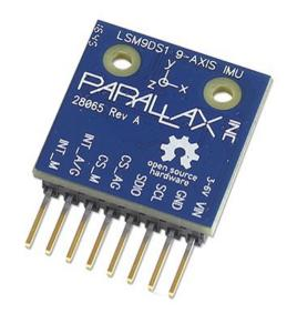
The LSM9DS1 9-axis motion sensor module can be used with nearly any microcontroller. It can be powered by 2.8, 3.3 or 5 volts and it uses either a 3-pin SPI interface or an I2C bus. Use it as a single sensor—accelerometer, a gyroscope, a magnetometer, or a temperature sensor—or all of the measurements can be read together for use in inertial measurement or dead-reckoning applications. It can also be configured to drive an interrupt when detecting impacts, free-fall, or magnetic field ranges.
