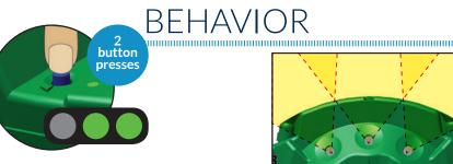
The three light sensors can detect bright light in front of the S3 robot. One sensor looks straight ahead, the other two look 30° to the right and the left.
