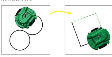
**NOTE:** Just like handwriting, each S3 drawing will be recognizable but unique every time you run a program. Variations occur as battery charge changes, motors warm up, and wheel joints relax with use over time.
