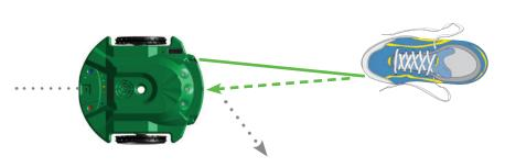
The S3's rear tail wheel is a stall sensor. If it get stalled on an object it cannot see, it will back up, turn, and try driving forward again.
