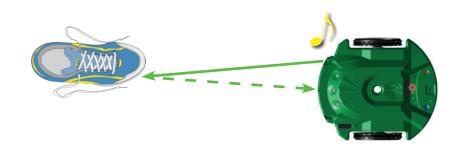
**EXTRA:** If the S3 can see the object with both sensors it will play both tones and both green LEDs will turn on. The S3 can see light objects better than very dark objects, because dark objects do not reflect much infrared light.
