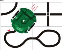
**EXTRA:** The S3 does best following black lines about 3/4 inch (2 cm) wide, on a white background. Line following works best when the track is placed on a hard, level surface. Carpet, tile, or other uneven surfaces may not work well. A dark surface may show through thin paper and make the line harder for the S3 to see.
