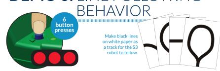
STEP 1: Print out a set of black lines from the "Tracks.pdf" (Download file from www.parallax.com/go/S3). Do not use photograph printing ink, which reflects infrared light!
