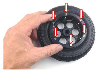
**Secure Rims - Aluminum Version:** Best practice for assembly is to get all of the screws started into their respective threaded holes. Then, tighten each one slightly and slowly go around the circle, which brings the two rim sections together evenly. Also, be sure to not pinch or bind the tube while screwing the assembly together.
