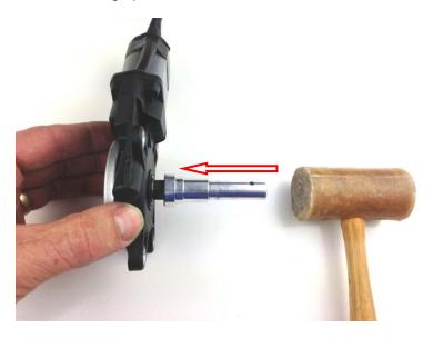
When the drive shaft is all the way on the motor drive pin, it should look like this. The distance between the motor housing and the large end of the axle should be approximately one-tenth of an inch.
