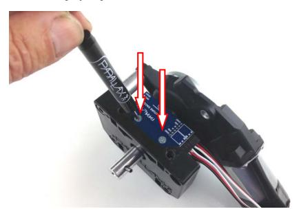
This completes the assembly of one of the drive units. Duplicate what you just accomplished and when you're finished the result is two separate motor drive units that are mirror images of each other—one for the right side and one for the left side of your robot platform, as shown here.
