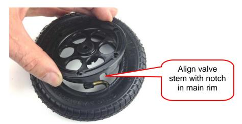
The aluminum wheel kit uses  $#4-40 \times \frac{1}{2}$ " long flat head bolts which screw directly into tapped holes on the aluminum Main Rim section.
