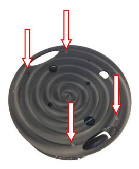
Step 3: (Optional) if you wish to add a second Top Deck, simply replace the four flat-head screws with the included 1.5" x 1/4"- 20 all-thread studs. Next, place the additional deck onto those studs, and then screw on the next set of standoffs. Place the second Top Deck onto that level and secure with four flat-head 1/4" x 20 screws.
