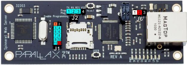
= VSS = VDD, 4 to 9 VDC = VIN, 3 to 3.6 VDC = I/O driven by VDD = I/O driven by VIN
