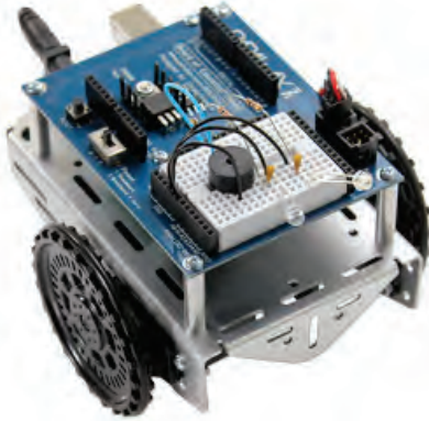
Board of Education Shield-Bot with Arduino Uno brain
