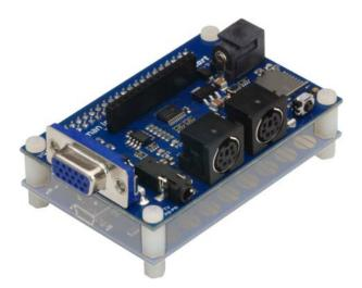
Connect the Human Interface Board to the QuickStart development platform before applying power. Power can be supplied through the USB port or the 2.1 mm center-positive barrel jack, or both at the same time. The QuickStart development platform can switch power supplies while it is in operation, although connecting the USB port to a host will cause the USB to serial converter on the QuickStart development platform to reset the Propeller chip.
