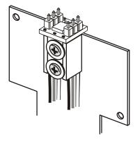
**Step 1:** Mount the HM55B Compass Module on the back side of the PING))) Mounting Bracket using (2)  $4/40 \ \frac{1}{2}$ " screws, (2) 4/40 nuts and (2) 10" servo extension cables.
