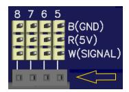
The top pin connects to Ground (Black wire). The middle pin connects to 5V, directly from the DC Barrel Jack (Red wire). The bottom pin (White) is the signal pin, and connects via an onboard 1K series resistor to the corresponding pin socket below (marked with the arrow).
