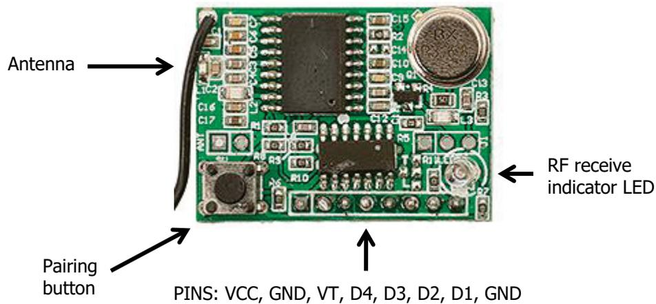
The Receiver Board has a pre-soldered antenna in "ANT2". To add even more range to the receiver you can add your own antenna to "ANT1" on the receiver board.
