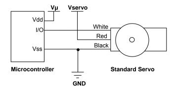
$V\mu$  = microcontroller voltage supply
