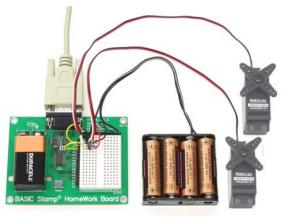
HomeWork Board with servo ports built on the breadboard, with a separate battery pack power supply for the servos.
