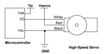
$V\mu$  = microcontroller voltage supply
