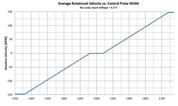
The rotational velocity response to tControl is fairly linear. This example graph is for 6.3 V, no load.
