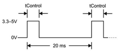
The duration (pulse width) of tControl determines servo rotation speed and direction as shown in the table below. The top speed will vary with supply voltage and load.
