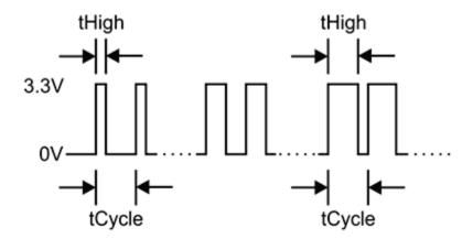
Duty cycle corresponds to the rotational position of the servo, in the units per full circle desired for your application.
