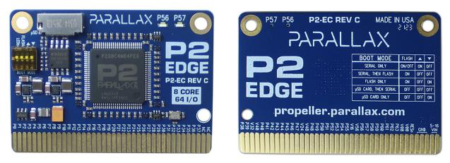
The P2 Edge Module is a simple way to get started with the Propeller 2 multicore microcontroller. In addition to speeding development, this module provides an optimal P2 building block for system integrators and designers to include in their products.
